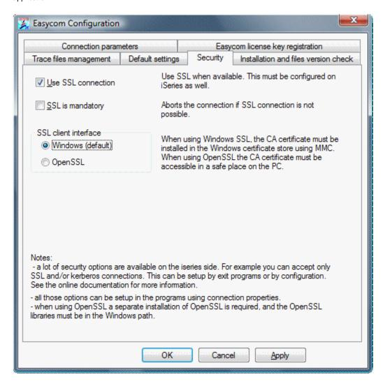
If SSL is activated, SSL connection will be attempted. If the SSL negotiation fails or not supported by the server or client, the connection will continue without SSL (not encrypted).
